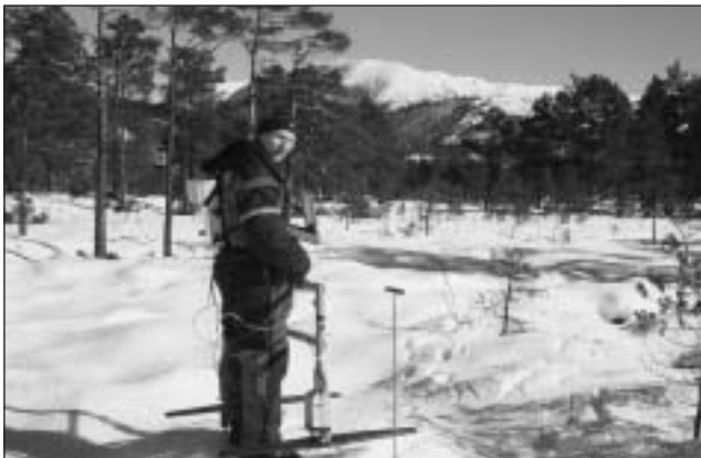
Fig. 10. GPR measuring for profile 1, Fig. 11 on the snow-covered bogs at Herlandsnesjane. Location: westernmost point on profile 1, Fig. 11.
